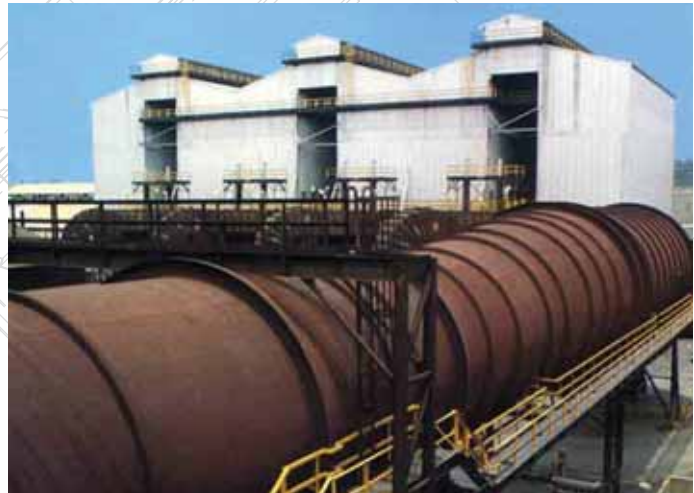
AmerTherm serving an EAF in USA. Flow: 2,700,000 m 3 /h
